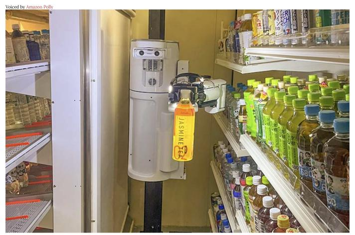
The TX SCARA robot is designed to work within the cold compartment of a convenience store and replenish stock 24/7. | Credit: Telexistence Inc.
