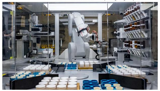
A-Lab, a facility at Berkeley Lab where artificial intelligence guides robots in making new materials. Photo credit: Marilyn Sargent/Berkeley Lab
